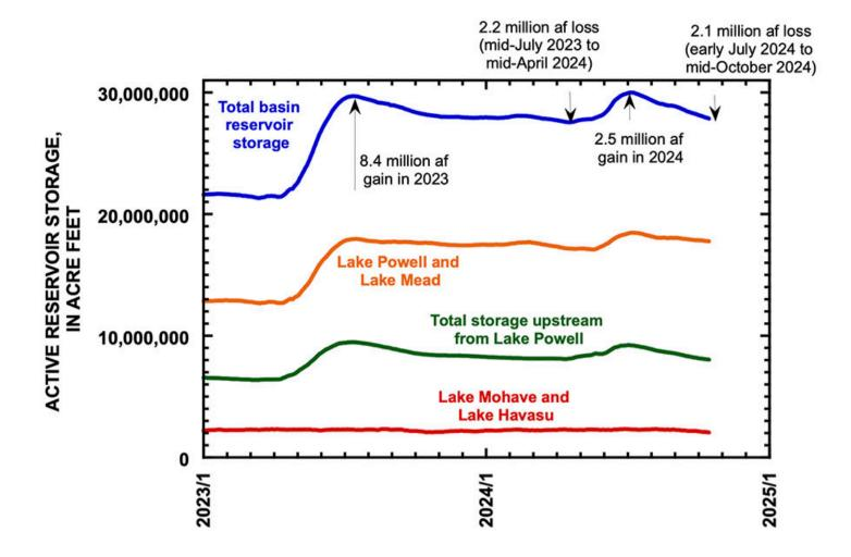
Figure 2. Graph showing reservoir storage between 1 January 2023 and 15 October 2024, highlighting the amount of reservoir recovery during each snowmelt season and the amount of reservoir drawdown during intervening periods.
