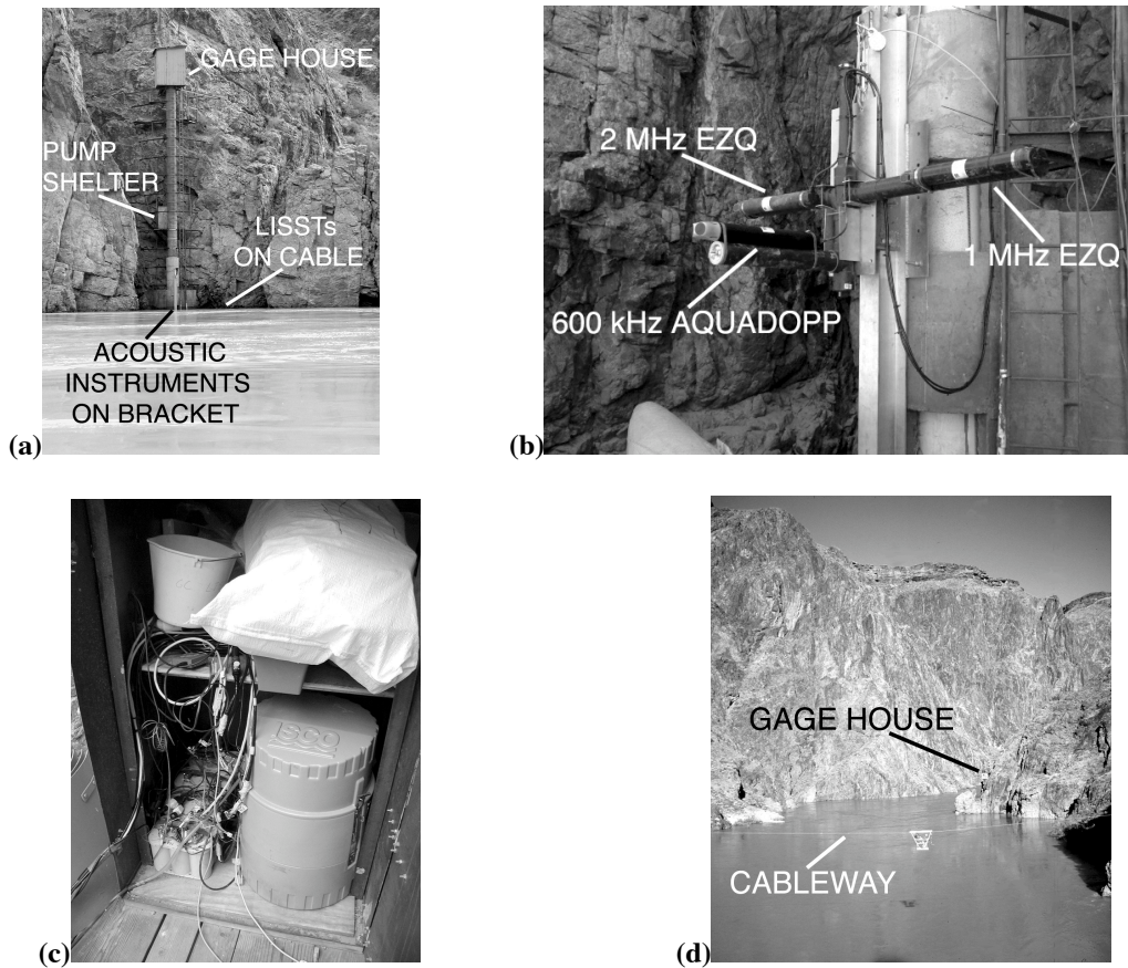
Figure 2. (a) Locations of instrument deployments at Grand Canyon gaging station. (b) Three-frequency acoustic-Doppler profiler array (out of water). (c) Contents of pump shelter in (a) showing automatic pump sampler (on right) and batteries. (d) Upstream view of reach showing measurement cableway and gage house in (a); cableway is 200 m downstream from gage house.
