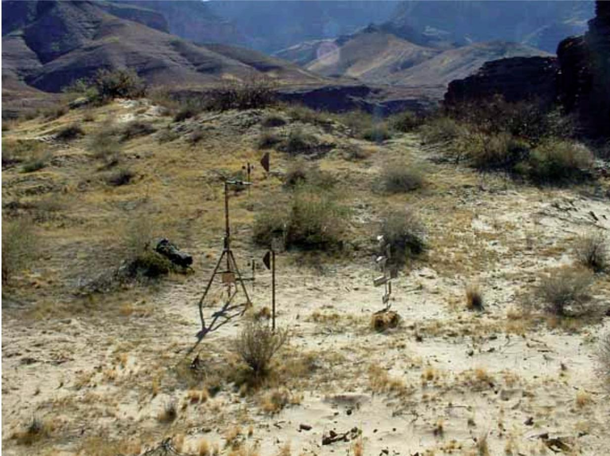
*Photograph of one instrument station. Four sand traps are shown on a vertical pole at the right of the photo. A tripod with two anemometers (at heights 2.0 m and 0.5 m above ground level) is at left; the data logger is also attached to this tripod. In the center is a tipping-bucket rain gauge. (click image to view a larger version).*
