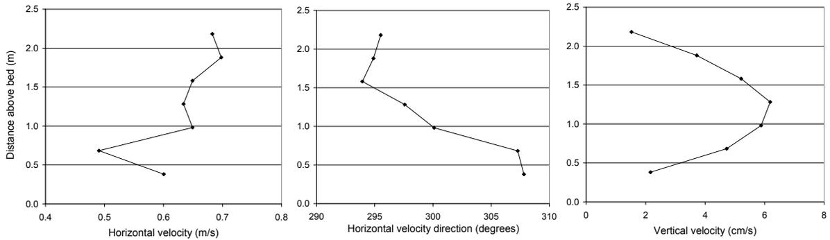
Figure 5. ADCP measured velocity profiles at station 3.
