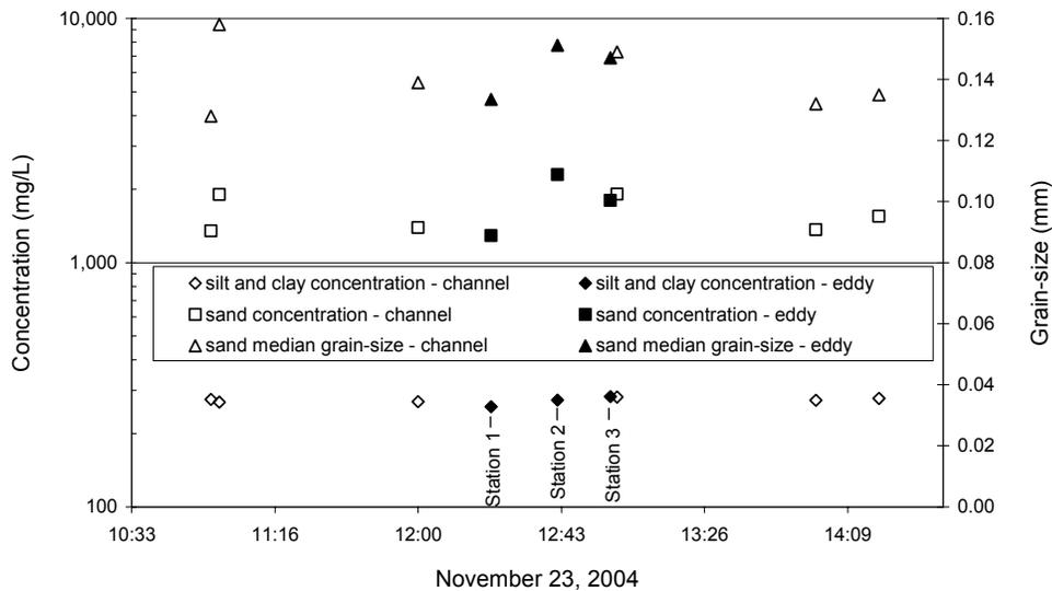
Figure 6. Measured silt/clay and sand concentrations and median sand grain-size in the main channel and at three locations within the recirculating eddy.
