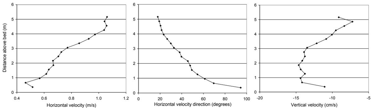
Figure 3. ADCP measured velocity profiles at station 1.
