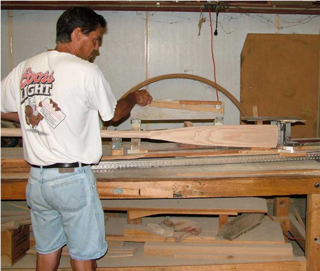
(Below Hoops Photos) 2007 Eric Swanson using powered blade cutter
