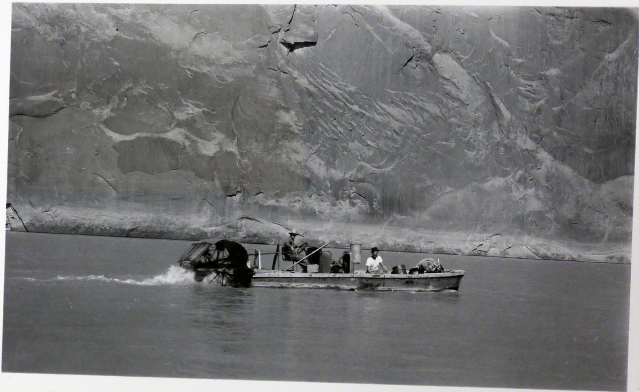
HUNT 899 1939 ART CHAFFIN'S STERN WHEELER ON COLORADO RIVER NEAR MOUTH OF BULLFROG CREEK. THE MOTOR IS FORD, MODEL A.
