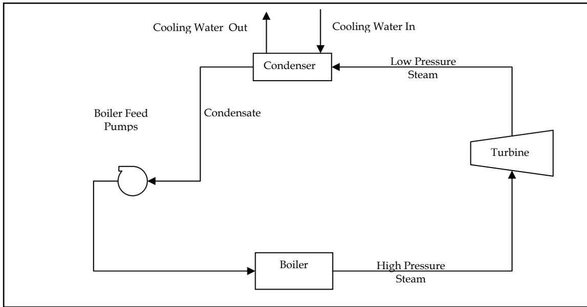
**Figure 1. Schematic of a Simple Steam Power Cycle**
