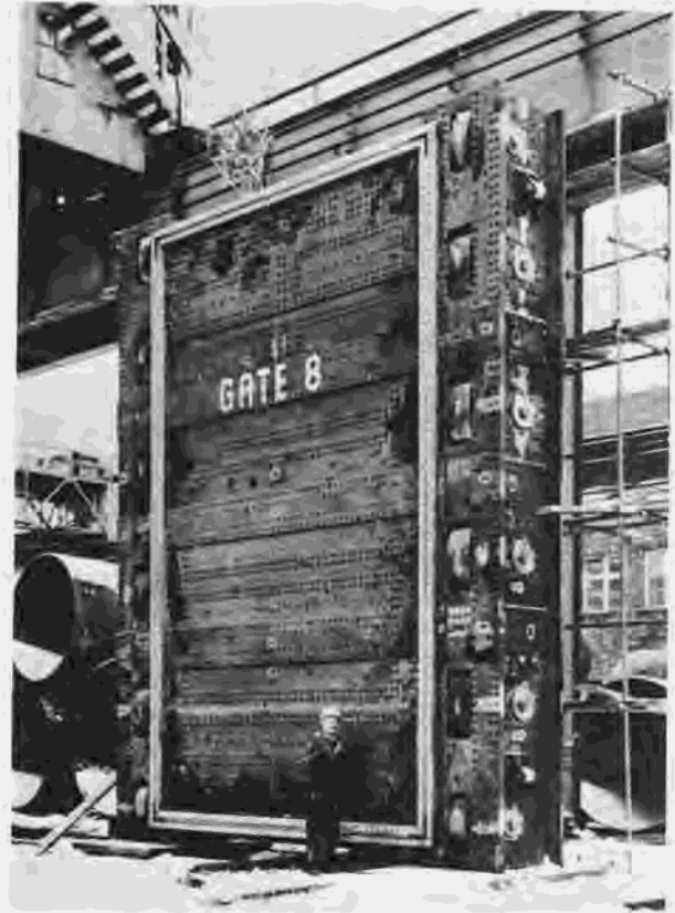
Figure 145.—Downstream elevation of shop assembly of 13.96- by 22.45-foot fixed-wheel penstock gate, P557-D-46362NA.
