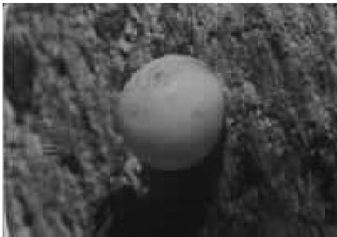
Figure 2 One of the earliest photos of alkali-silica “gel” common to expansive alkali-aggregate reaction. These gels swell in the confined concrete matrix causing expansion and cracking in the aggregates and concrete. Bureau of Reclamation Concrete Laboratory file photo, about 1940.
