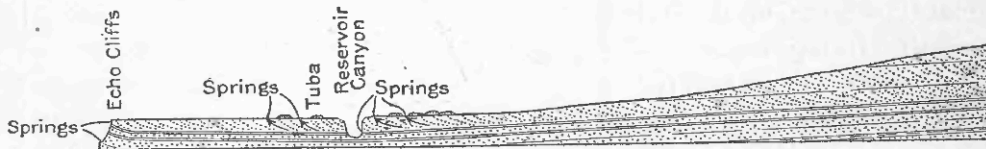
FIGURE 17.—Section across Kaibito Plateau, illustrating the conditions which determine the distribution of springs at Tuba.
