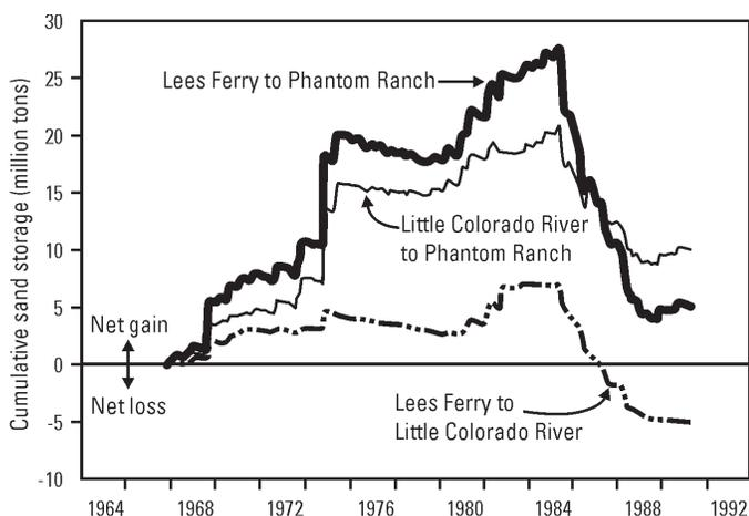
**Figure 2.** Reproduction of figure III-15 from the final environmental impact statement (EIS) (U.S. Department of the Interior, 1995), which shows the sand budget as computed by Randle and Pemberton (1987). Recent studies refute the conclusion of the EIS that sand accumulates on the bed of the Colorado River over multiple years under normal dam operations. (Phantom Ranch is the location of the Grand Canyon gage.)
