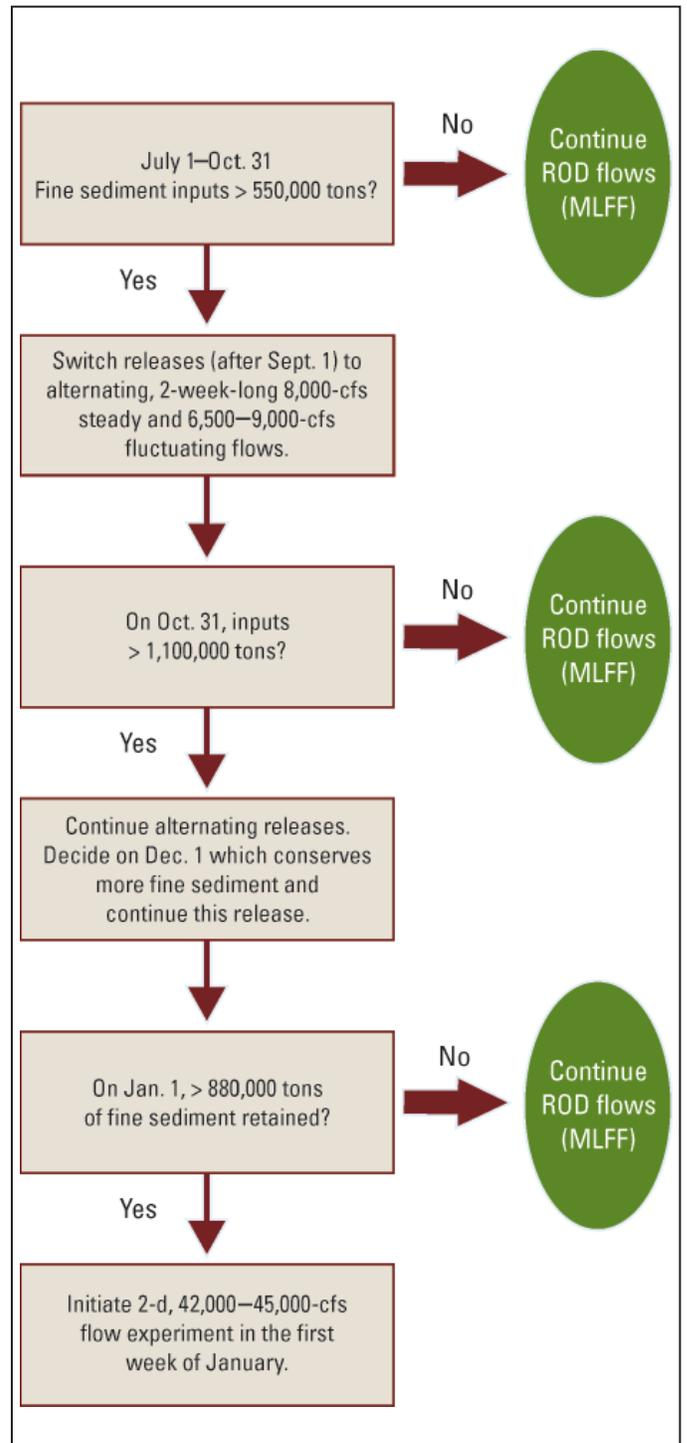
**Figure 9.** Sequence of events established in the autumn sediment input scenario in an environmental assessment by U.S. Department of the Interior (2002) related to fine-sediment inputs and retention to trigger a 2-d, 42,000–45,000-cfs experimental high flow in January. If fine-sediment inputs do not reach specified levels, then modified low fluctuating flow (MLFF) operations, as specified in the Record of Decision (ROD) (U.S. Department of the Interior, 1996), are continued.
