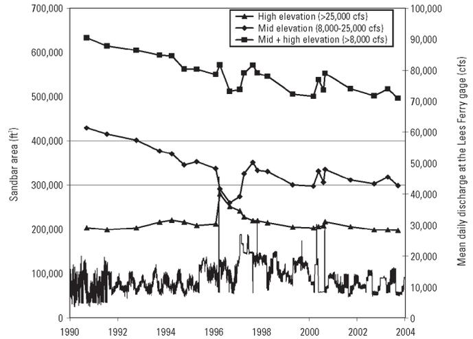
**Figure 6.** Changes in sandbar size (total surface area) are shown for 14 long-term sandbar study sites between the Lees Ferry and Grand Canyon gages (RM 0 to RM 87). Area of bars exposed above water discharges of 8,000 cfs decreased by 22% from 1991 to 2004. The 1996 beach/habitat-building flow resulted in a net transfer of sand from mid elevations to high elevations (modified from Rubin and others, 2002).
