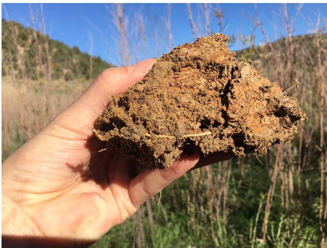
Figure 49: View of soil sample for Wetland 2 showing redox depressions.
