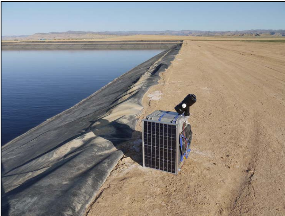
Figure 3. Bat detector high frequency microphone and recorder, programmed to make night recordings.
